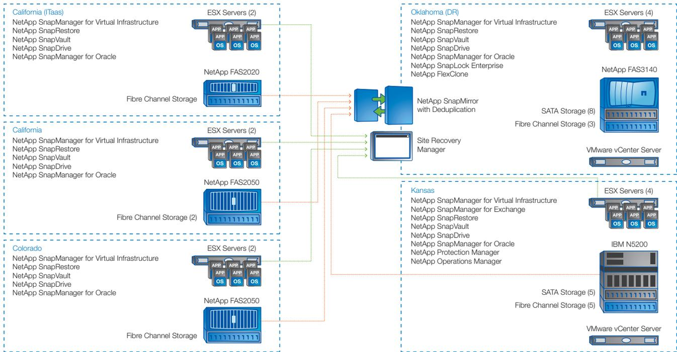
**Figure 1. DCI leverages more than 100TB of NetApp storage across five data centers. NetApp storage complements the DCI VMware environment to deliver cost savings, data and business protection, plus cloud-enabled IT service delivery. Benefits include: within-minutes, automated DR; reduced power/cooling costs; the ability to manage >100TB with just one FTE; and a technology foundation for business agility, innovation, and competitive advantage.**
